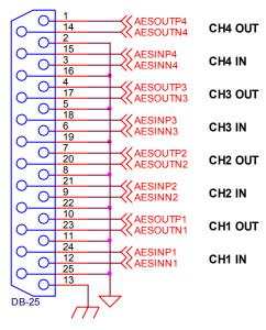
ANALOG AUDIO - INPUT & OUTPUT PINOUTS ARE IDENTICAL
